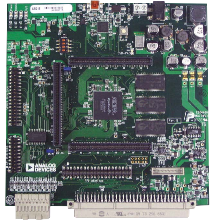
FIGURE 5. Reference design boards provide support circuits and communications that let you test an ADC.
